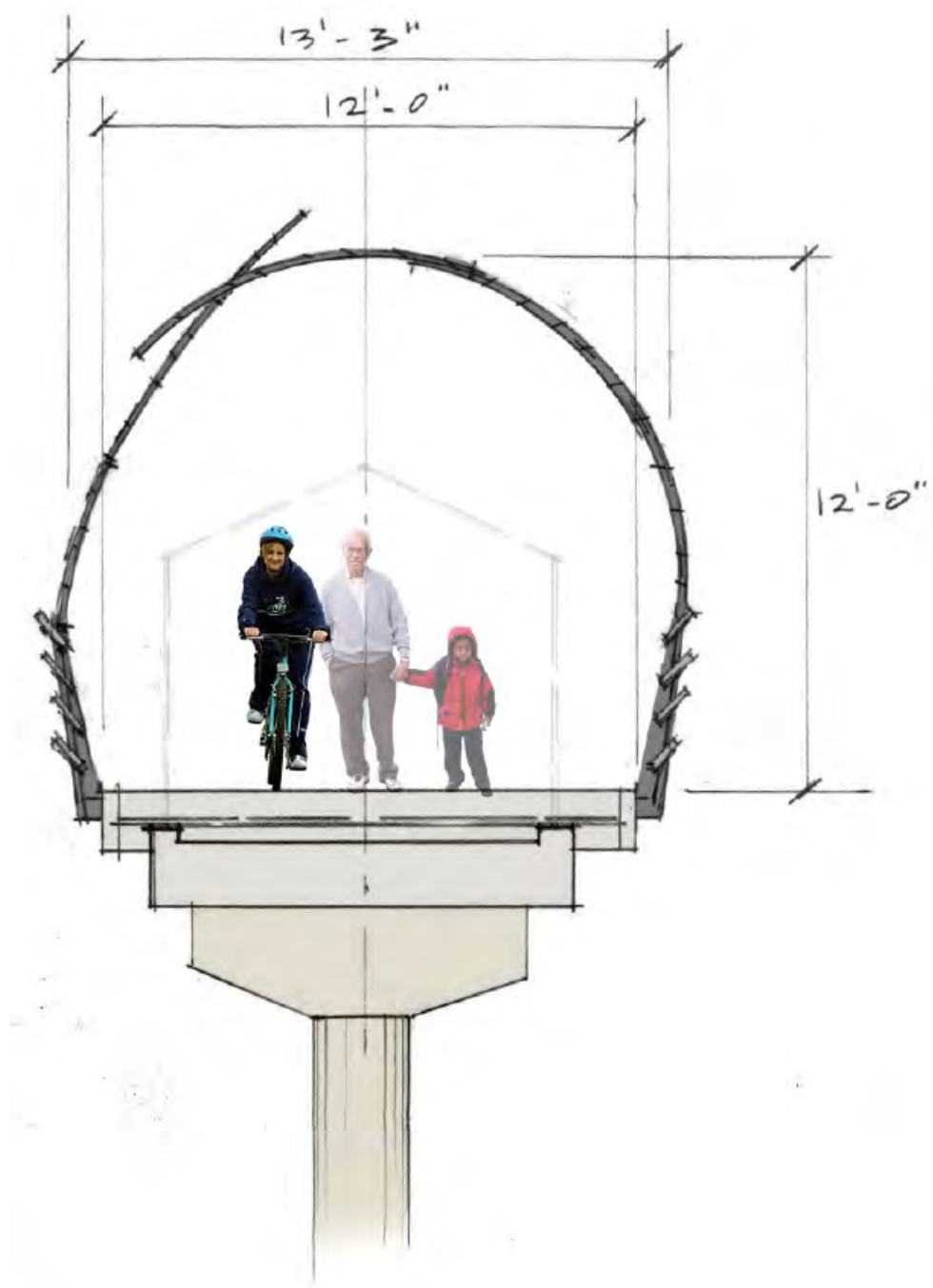
Option 2 Bridge Section - Place new deck with 15" cantilever on top of existing bridge deck. 12'-0" clear to overhead fencing.
