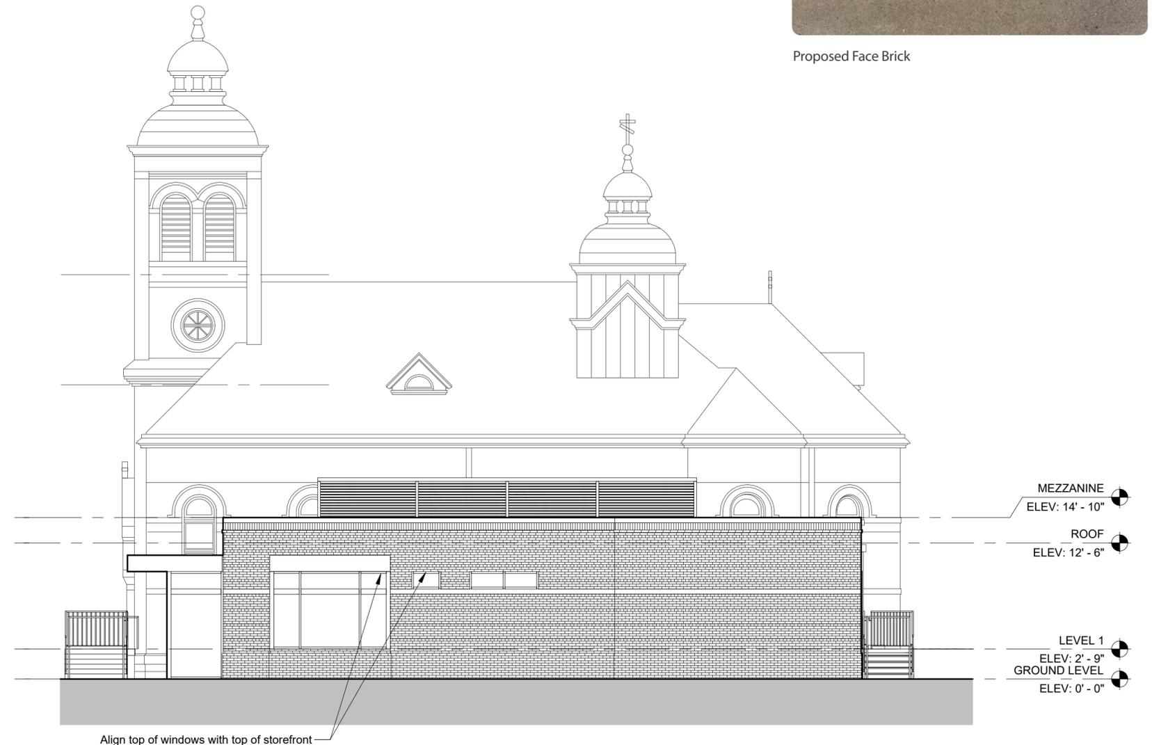
Note: Design intent is for all horizontal bands on the church to align with the corresponding bands on the addition.
