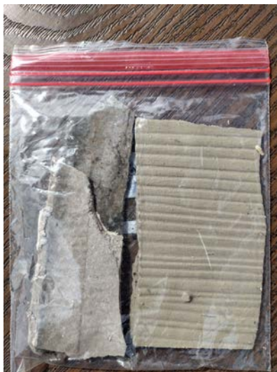
Transite Siding shingle sent to lab contained asbestos.
