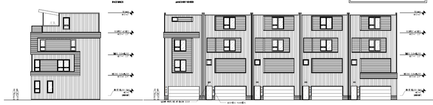
4 BUILDING 2 - WEST ELEVATION SCALE: 1/8" = 1'-0"
