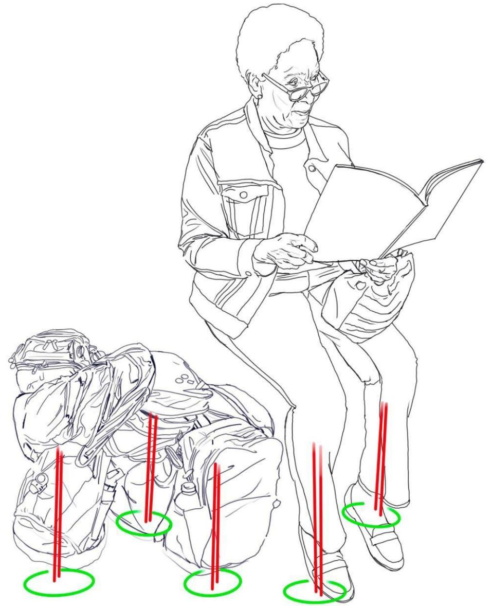
**Steel rods connect sculpture to concrete poured underground**
