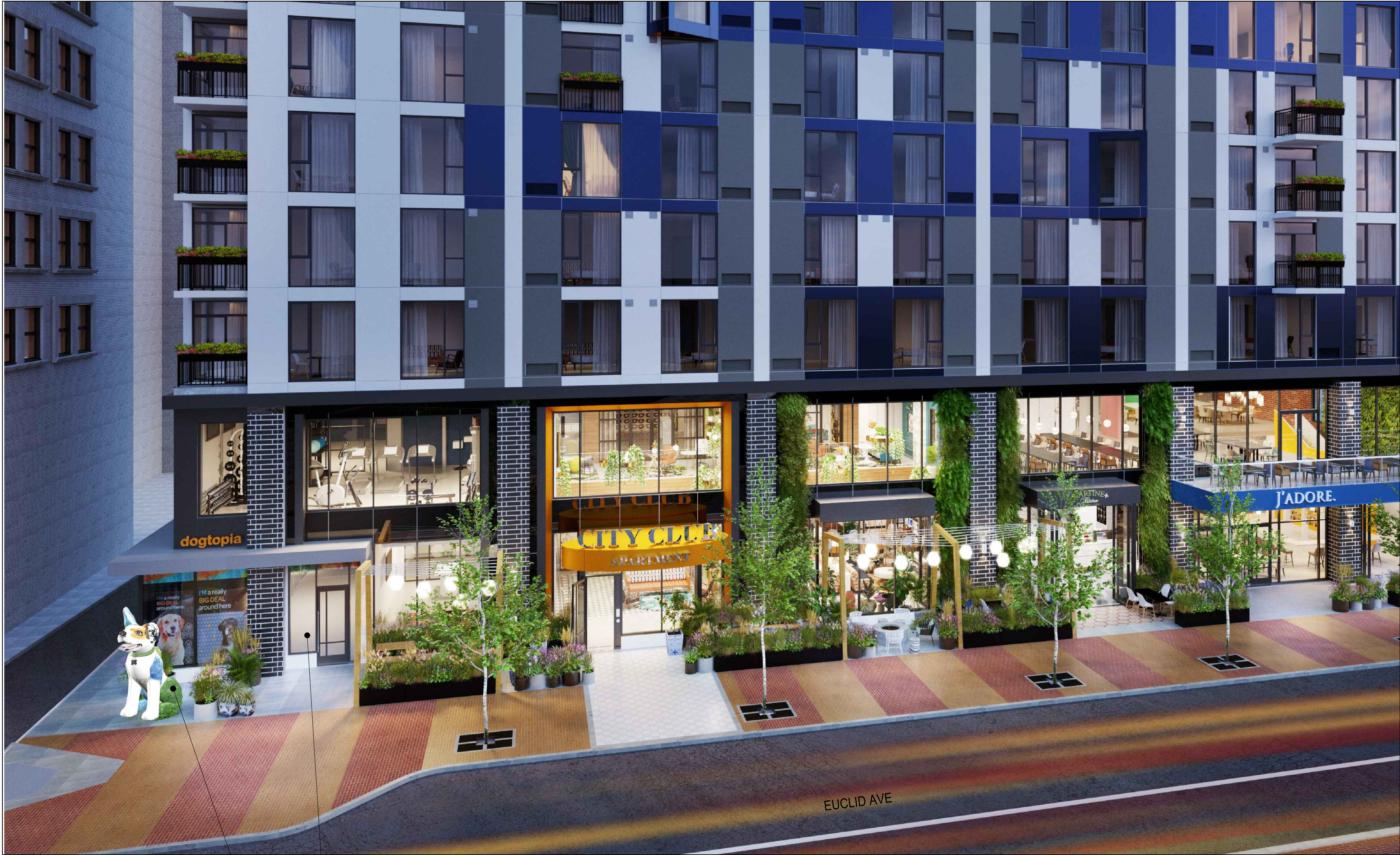
DOGTOPIA 10' HIGH SCULPTURE MADE OF HIGH DENSITY FOAM ON ALUMINUM FRAME WITH POLYURETHANE, POLYUREA HARD COAT AND FINISH COAT
