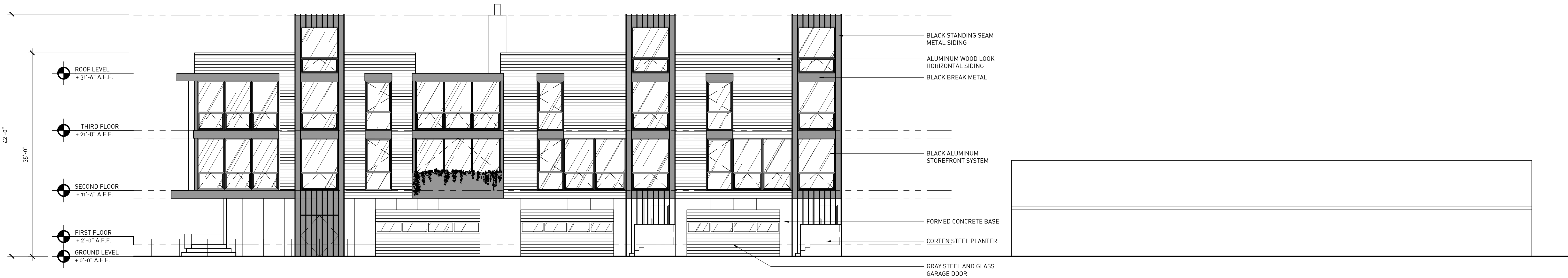
4 83.1 NORTH ELEVATION SCALE: 1/8" = 1'-0" REQUIRED FIRST-STORY GLAZING - 85 S.F. PROVIDED FIRST-STORY GLAZING - 100 S.F.
