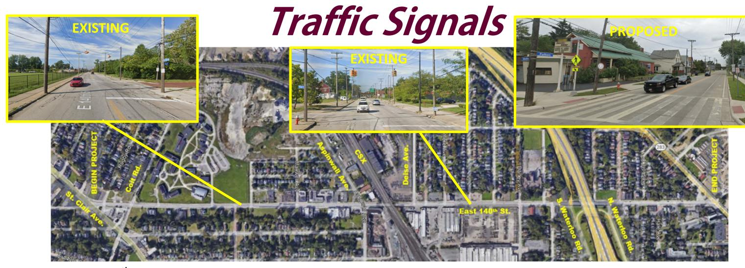
East 140<sup>th</sup> & Nell Avenue: Remove overhead beacons and replace with FYG signage and RRFBs on 140th.
